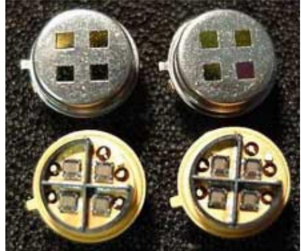
Figure 5: The quad thermopile sensor TPS 4339 houses four thermopile chips in a single TO 5 case. The open detectors in the lower row show clearly the internal aperture, that suppresses successfully any crosstalk between the four channels. Even this sensor type employs a thermistor (the small cube in the upper right position) to provide an internal temperature reference. The upper row shows closed sensors carrying four different IR bandpass gas filters.
